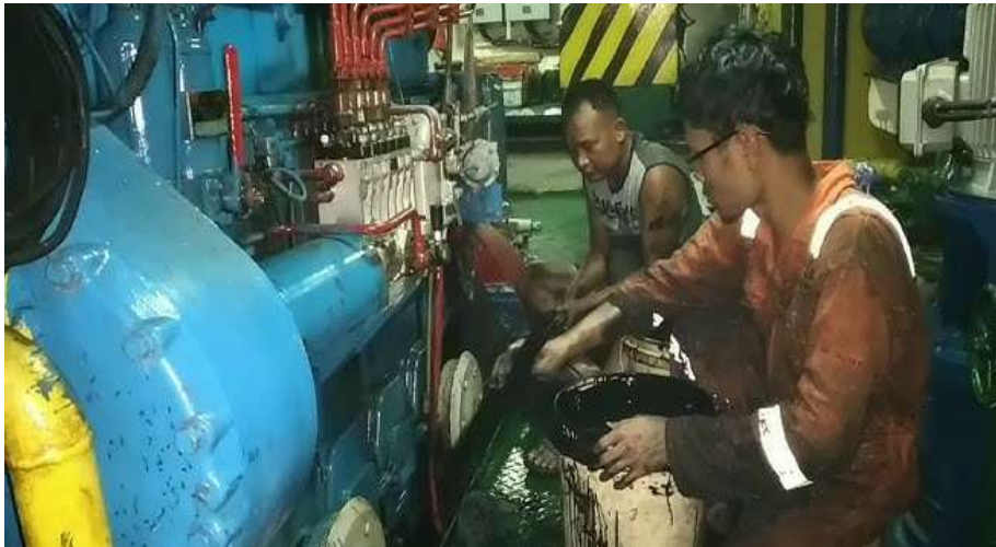
Figure 1. Lubricating Oil Filter Replacement in the main machine
