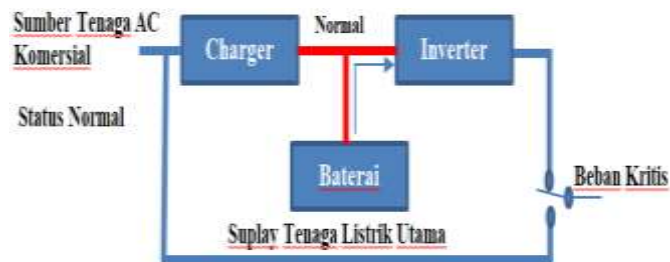
Figure 3. Reverse UPS System
