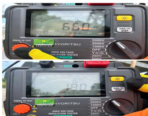
Figure 5. Results of S Phase Testing (Primary – Ground)
