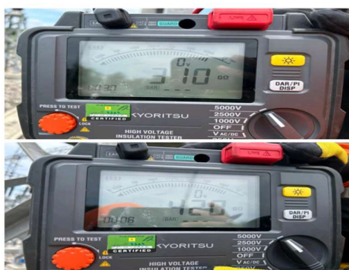
Figure 7. T Phase Test Results (Primary – Ground)
