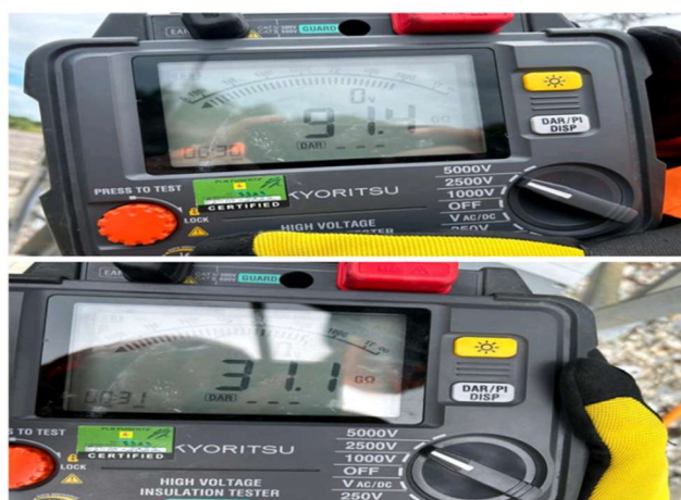
Figure 3. R Phase Test Results (Primary – Ground)
