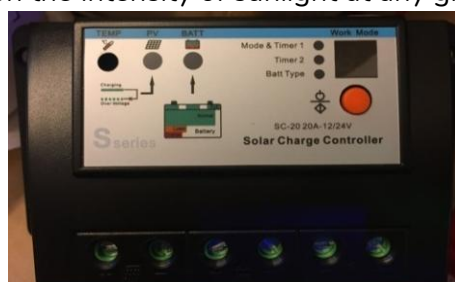
Figure 4. Solar Charge Controller (SCC)
