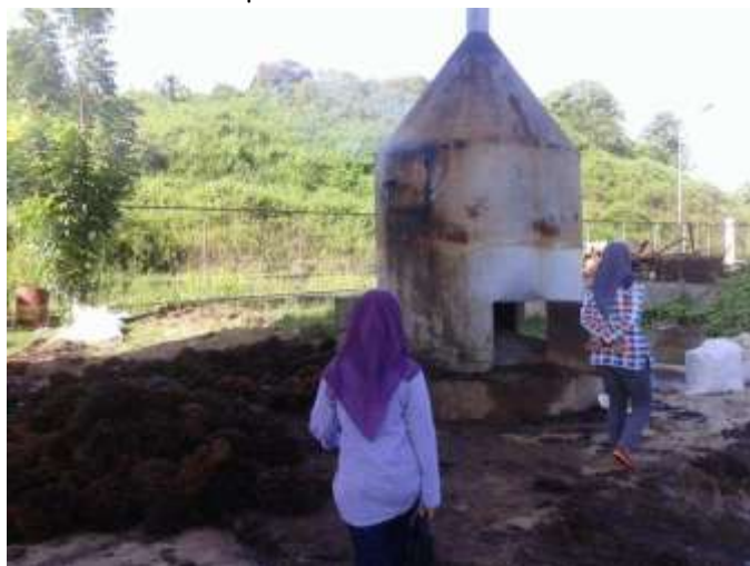
Figure 2. Oil palm empty bunches burning furnace
