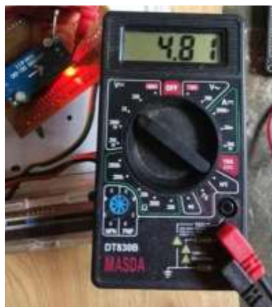
Figure 10. Measurement results of 5 Volt DC voltage that has been reduced
