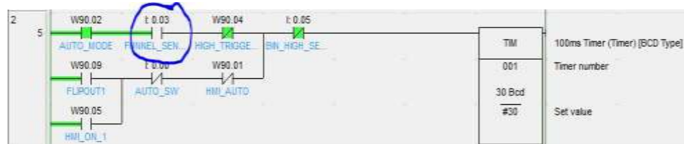
Figure 9. Ladder Diagram of Intake Sensor
