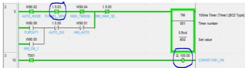
Figure 10. Ladder Diagram of ON Conveyor Machine
