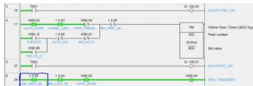
Figure 13. Ladder Diagram High Level ON
