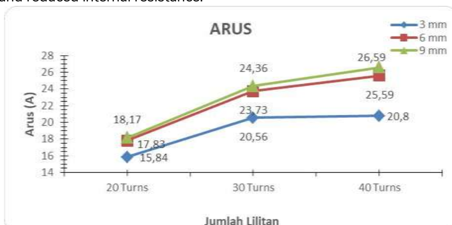
Figure 4. The Effect of Changes in the Number of Turns on the Current Value
