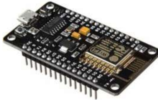
Figure 3. ESP8266, One of the popular microcontrollers for IoT
