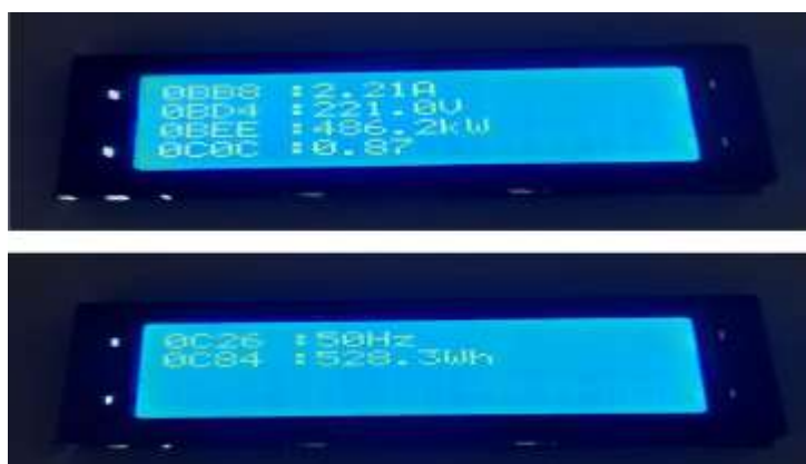
Figure 9. Energy Meter Testing
