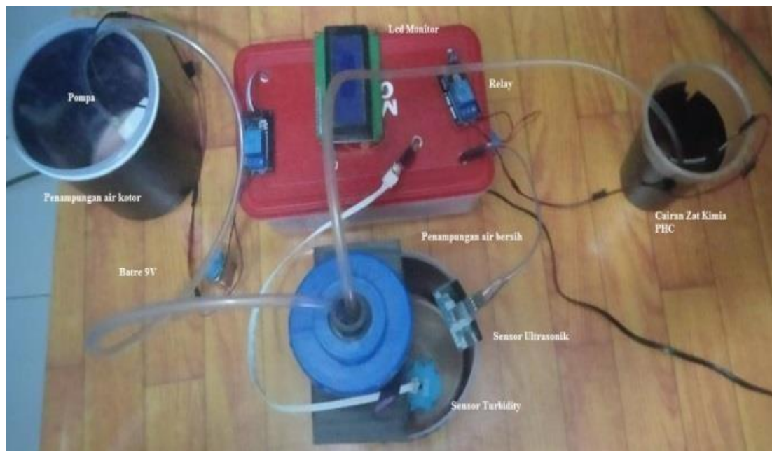
Figure 5 Results of Water Depth and Turbidity Monitoring System Design
