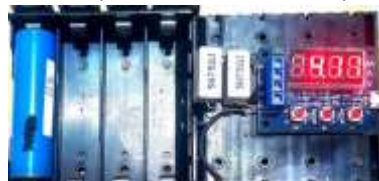
Figure 14. degradation of battery by sculpting module HW-586/Zhiyu battery capacity meter Source: Personal documents
