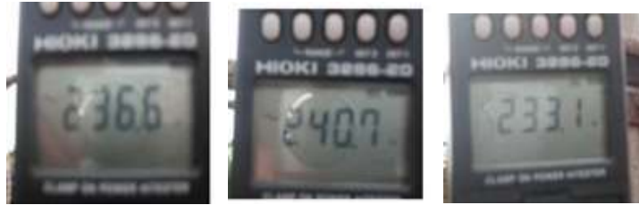
Figure 8. Output Measurement Documentation Joint Press Connector Connection Point (a) RN (b) SN (c) TN
